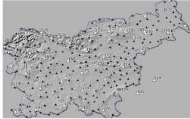
Figure 14: Trigonometrical net of first order in Slovenia
